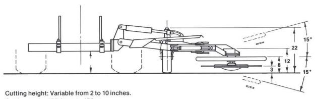
Cutting angle: 15° down to 15° up. Hydraulics required: 8 GPM. Shipping weight: 582 pounds. Blade diameter: 31 inches.
