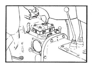
Edwards offers a variety of tractor hydraulic manifold plates to make pressure and return ports available for operating various implements and attachments. Edwards has developed these manifolds to adapt Edwards Forklifts, Front 3-Point Hitches, Brush Spiders, Highway Mowers and other hydraulic actuated implements. For instance, with the TF575 Manifold Sub-Plate shown here, any number of valves can be added to older Ford 600-800 up to current Ford tractor models.
