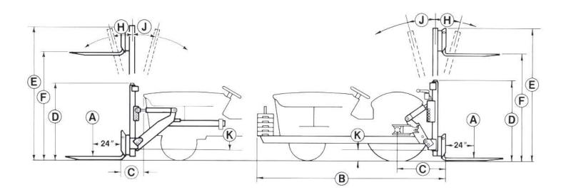
FORKS: Forks are made from 1<sup>1</sup>/<sub>4</sub> x 4 heat treated alloy steel. Standard length is 46". Standard carriage width is 29 inches. Fork spacing is adjustable. Other fork lengths and carriage widths are available on special order.
