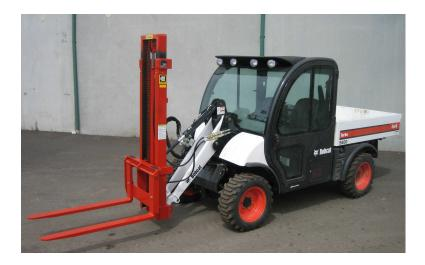
The TRANS-TIER is made from high quality materials. Sealed ball bearings support the fork carriage. The slide channels are a special section rolled from high carbon steel. Hard chromed rod is used in all hydraulic cylinders. A rugged mounting bracket attaches the TRANS-TIER quickly and easily to the Available 120 and 144 loader frame. inch lifting heights.
